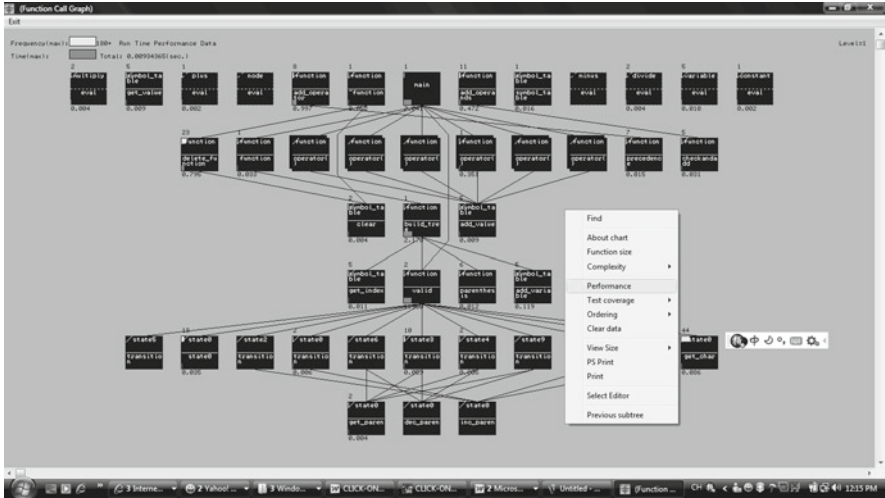
Fig. 1.5 View the performance measurement result for locating bottlenecks (a bar at the bottom of each module-box shows the percentage of the time used)
